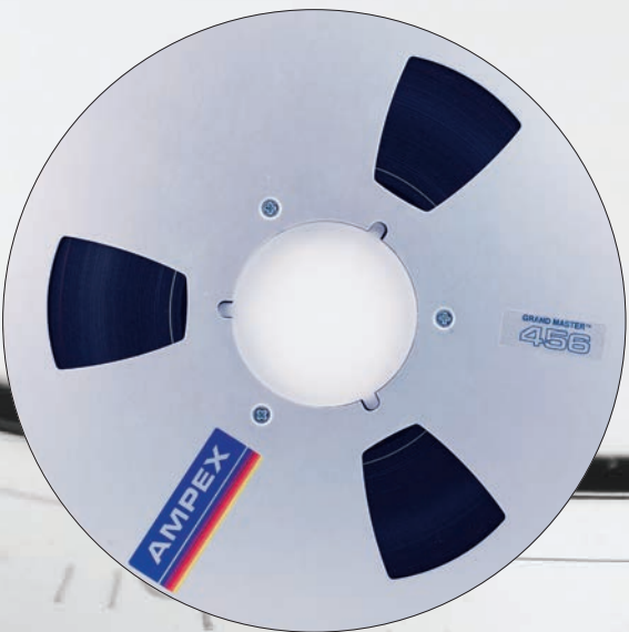
▼ 'Strategy' 10" master tape reels. The Ampex tape (left) contains the A side of the album and the Scotch tape (right) the B side. Both reels are wound 'tails out', meaning the start of the recording is nearest the centre of the reel. The Ampex 456 tape has replay alignment tones (notes sounded at various frequencies) before the recording begins. They were last played in 2017 and remain in excellent condition.
